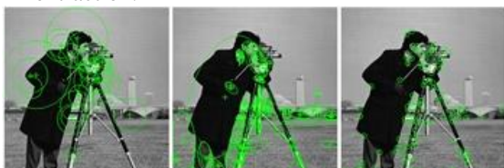
Fig2.1 SURF (left), MSER (center), and corner detection (right) with Computer Vision System Toolbox. Using the same image, the three different feature types are detected and results are plotted over the original image.
